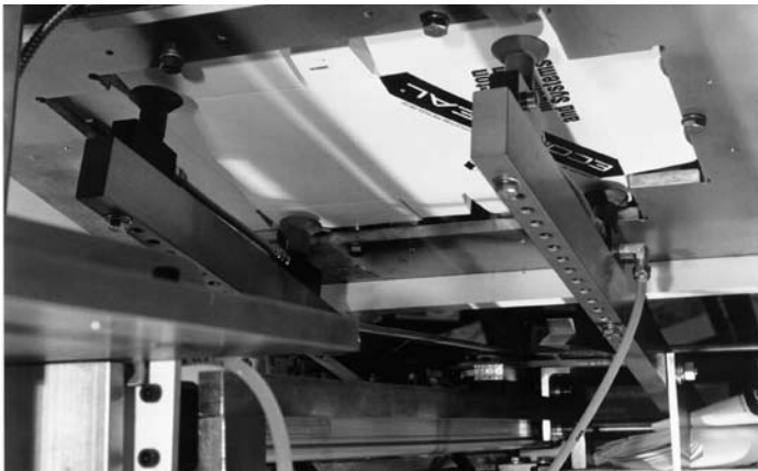
Flat Blank is automatically pulled from a supply magazine with vacuum cups and transported to the forming area.
