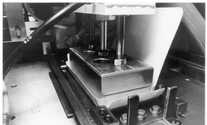
Mandril plunges blank through tooling cavity and the result is a completed corner glue, cornerlock, or simplex tray.
